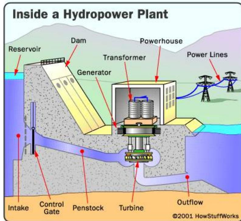
In hydropower, water is piped from the river and will rotate the propeller turbine and generator to produce electricity. Wires to large cities transmit electricity. In environment, water runs rampant and the strength of current produces the necessary pressure. Hydroelectric water is stored in reservoirs created by the dams and then used as necessary.
